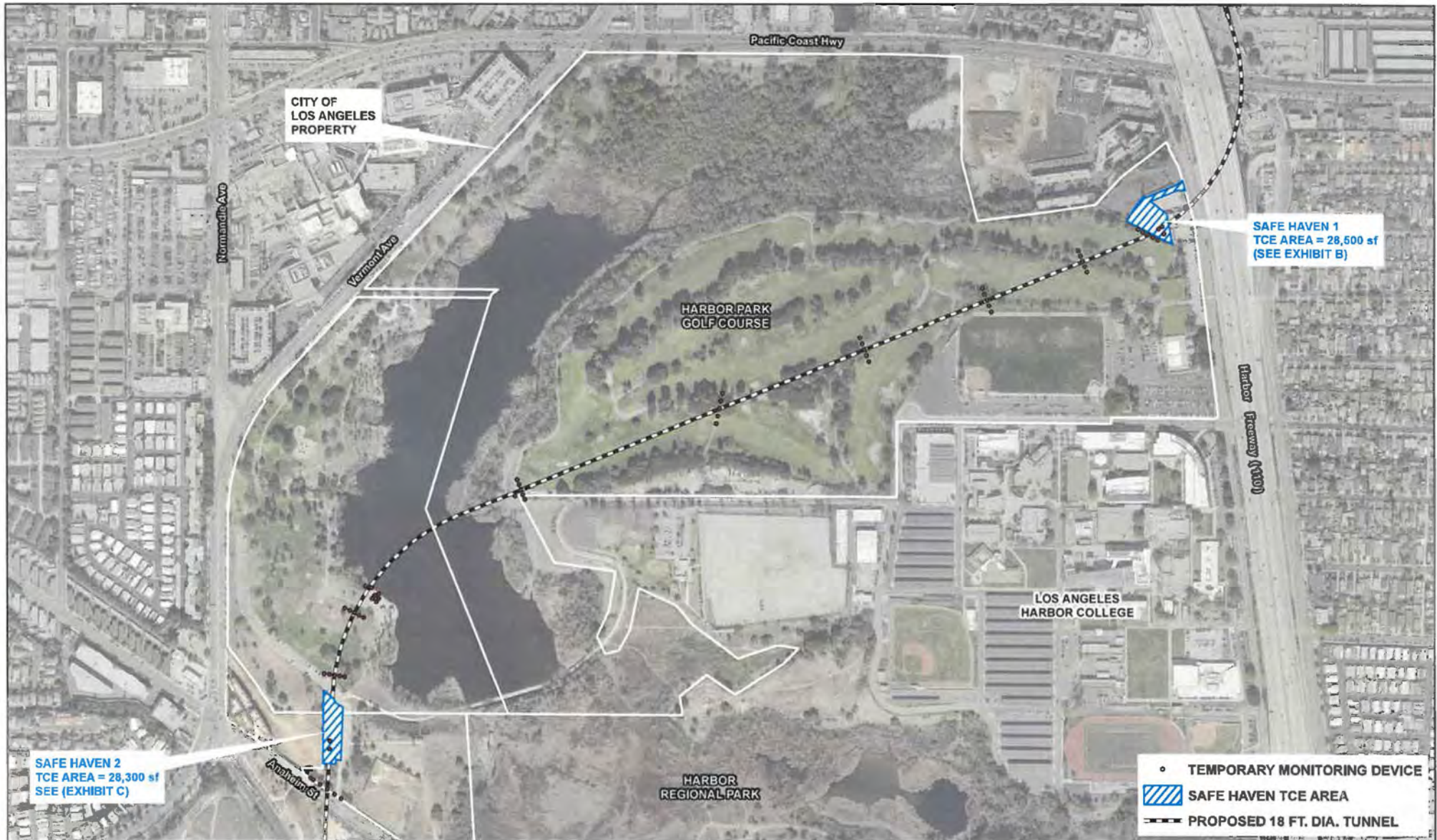
Exhibit A JWPCP Effluent Outfall Tunnel Project - Temporary Construction Easement Areas for Safe Havens (Up to 6 Months) and Temporary Construction Easement for Monitoring (Up to 18 Months)
