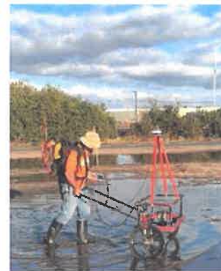
EM-61 Data acquisition
