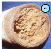
PROBLEM: GALVANIZED IRON WATER SUPPLY PIPES ARE CORRODED
